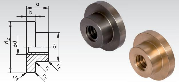
Ordering Details: e.g.: Product No. 644 010 00, round flange nut made from GG25, Tr. 10 x 3, single thread, right hand
