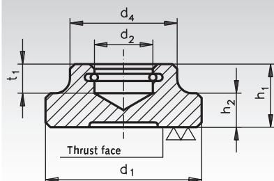
Ordering Details: e.g.: Product No. 654 106 00, Thrust Pad DIN 6311, d<sub>1</sub> = 12 mm
