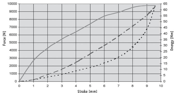
With aid of the characteristics curves above you can determine the amount of the energy that will be absorbed.
