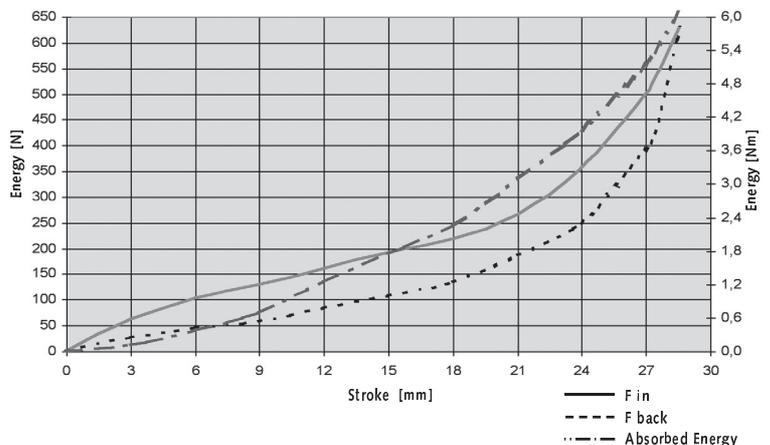
With aid of the characteristics curves above you can determine the amount of energy that will be absorbed.
