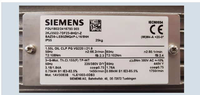
Fig. 12/4 Example, rating plate on the motor
